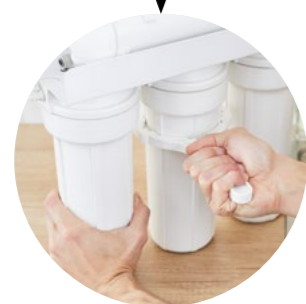
Maintenance and cleaning of the water filter
